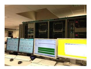
The objectives of this testing facility are mainly to study adverse control interactions and test multi-vendor and multi-infeed schemes. It is also used to validate the various modeling approaches for a large range of different phenomena, and to support maintenance activities.
