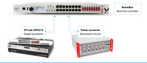
Users can use all six half-bridges to implement back-to-back converters, such as grid-tied var-speed drives, HVDC systems, etc. Alternately, fewer modules may be sufficient for applications such as PV inverters, battery chargers, etc.
