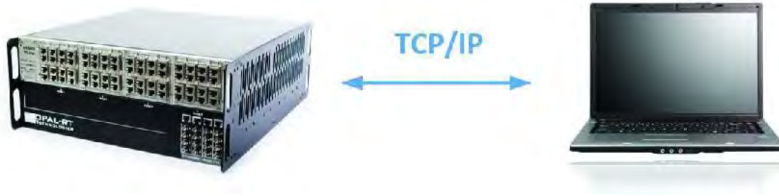
Figure 7: Real-Time Simulator (Target) and Windows Command Station (Host) Communication
